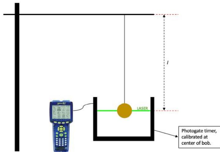
*Fig. 1 – A side view of the apparatus*
