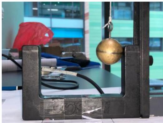
*Fig. 2 – An image depicting the vertically calibrated bob (against the photogate). It was horizontally shifted for conducting oscillations.*
